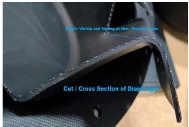
Diaphragm Cut Section
