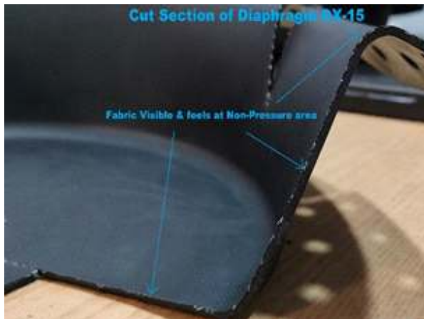
Diaphragm Cut Section
